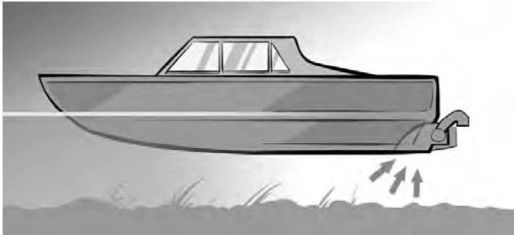
Figure 8. Suction power of the intake
