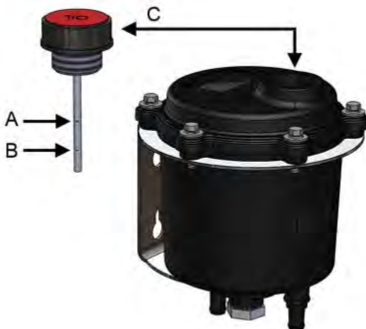
Figure 22. Checking the oil level
