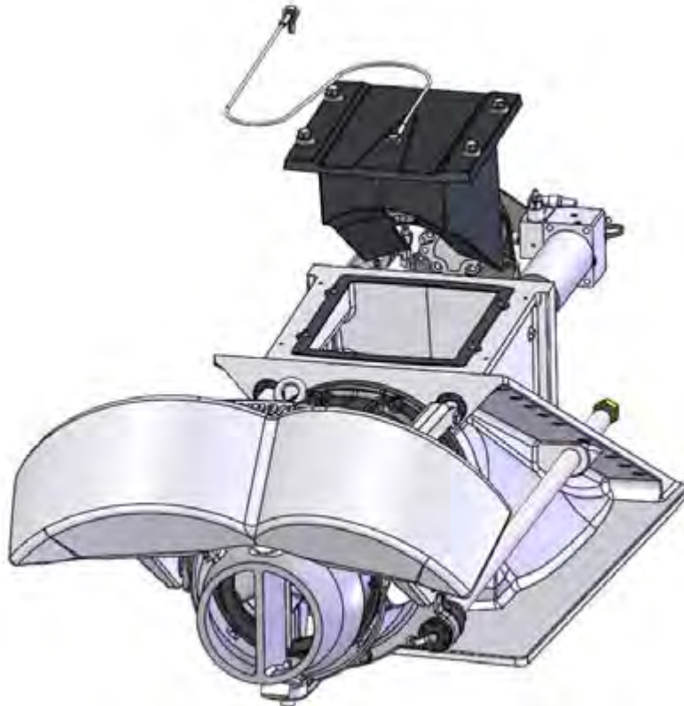
Figure 41. Opened inspection hatch
