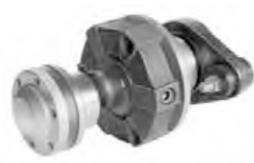
Figure 55. Intermediate shaft with rubber stop
