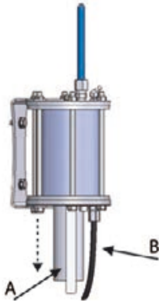
Figure 23. Automatic lubrication unit's piston movement range
