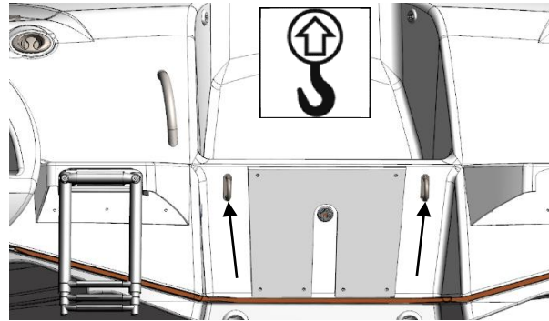
Fig. 29. Rear lifting eyes, 2 positions.
