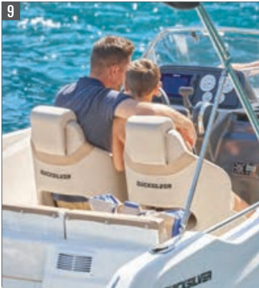
Pilot & co-pilot bucket seats with flip bolster and swivel, pivoting seats. New seat design as of MY2019 not shown in brochure.
